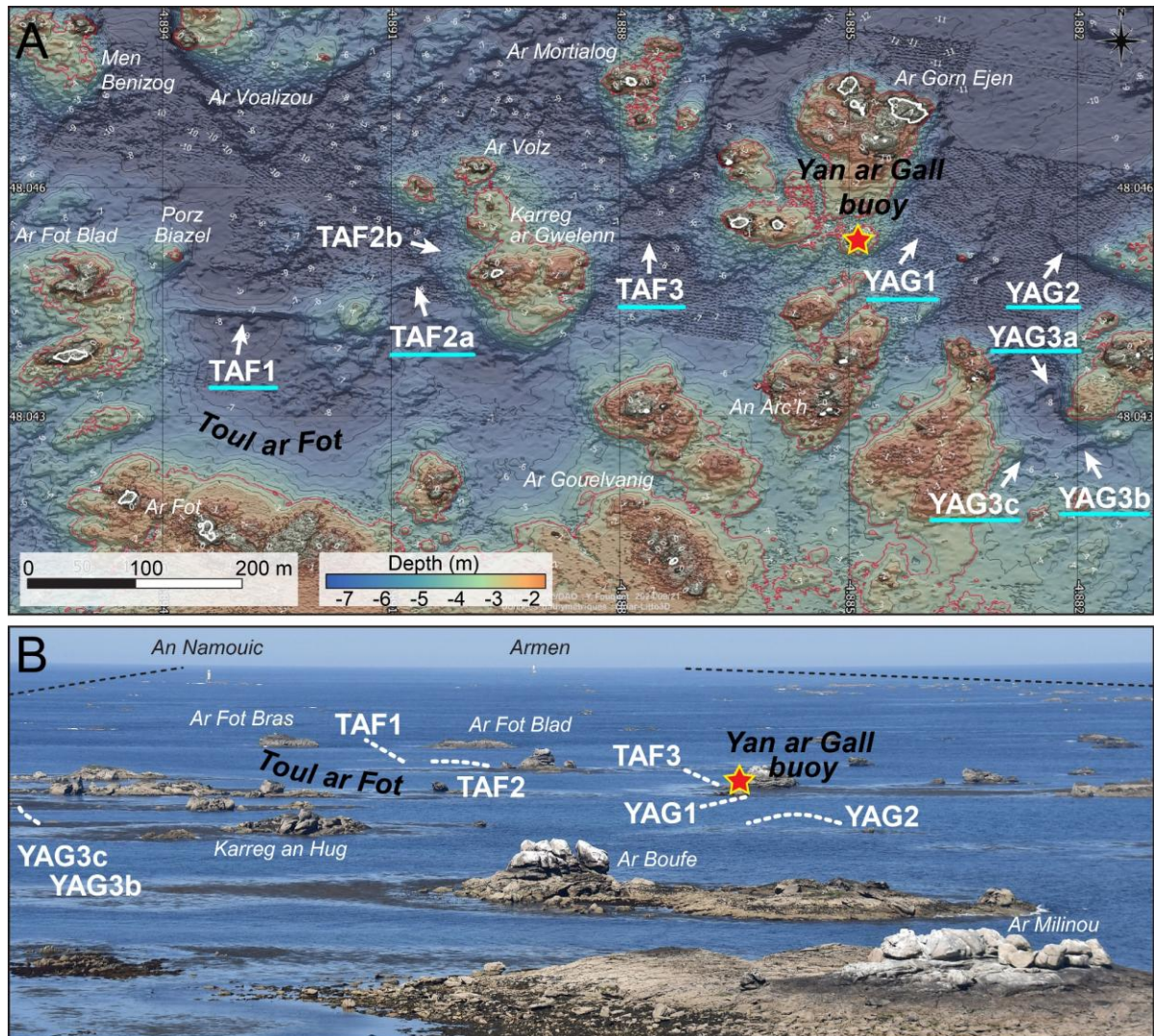
Figure 2. Toul ar Fot and Yan Ar Gall sectors. A: Bathymetric map and position of the Toul ar Fot (TAF) and Yann ar Gall (YAG) structures. See Figure 1 for the location of the map. Black elevation contours are spaced 0.5 m apart. Depths on the curves are given in metres above sea level (asl). The current coastline (thick white curve) and lowest astronomical tide level (red curve) are also displayed. The names underlined in turquoise blue indicate the walls that have been explored by dives. B: Panoramic view taken from the top of the Sein Island lighthouse, showing the reef line of Sein (see Figure 1) at low tide. The northern and southern boundaries of this granitic plateau are indicated by the gray dotted lines. The position of the structures explored during the dives is indicated by their name and by the white dotted lines. The names of the lighthouses and navigation towers are indicated in black (Authors).
